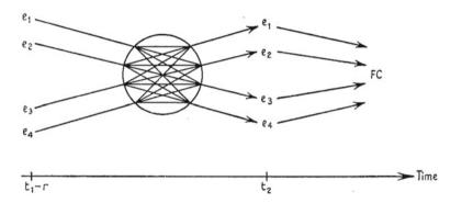
**Fig. 17.2** The same scheme as in Fig. 17.1 except that the nerve connexions have been centralized (within the *circle*), showing the great economy in the overall length of the communication channels (see text for further explanation) (after Sommerhoff 1950; reproduced by permission of Oxford University Press [Fig. 9, p. 131])
