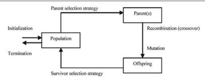
**Fig. 8.1** An example of a genetic algorithm. One complete cycle constitutes one generation. Survival selection strategy determines which offspring, and which parents, are allowed to pass through to the next generation and which of those are allowed to become parents in the next cycle
