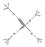
**Fig. 11.1** A water molecule hydrogen-bonded to its congeners. The hydrogen atom is typically 0.10 nm from the oxygen to which it is covalently bonded (*solid lines*) and 0.18 nm from the neighbouring oxygen to which it is hydrogen-bonded (*dotted lines*). The energy of the hydrogen bond (H-bond) is about 0.1 eV (i.e., about  $4k_BT$  at room temperature or about 2.4 kJ/mol)
